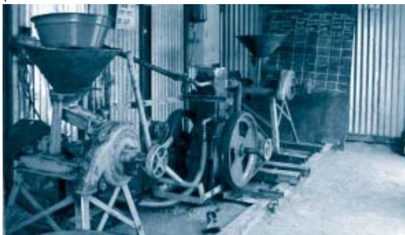
Multifunctional platform mounted with food processing devices.
